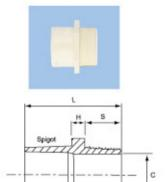
The spigot end of this fittings is solvent cement jointed to the socket of another fittings. The tapered male threaded end provides a connection for PVC, brass or galvanised wrought iron threaded valve-Type fittings.
