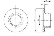
Flanges are used to bolt PVC pipes to pumps and valves etc. Flanged disconnectable fittings provide capability for maintenance and future changes to the pipeline.
