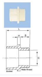
The valve socket is solvent cement jointed to a pipe spigot. The malethreaded end of the valve socket provides a connection for a PVC, brass or galvanised wrought iron threaded-type fitting.
