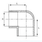
These are moulded fittings, which are used to provide  $90^\circ$  bends in pipelines. They are often employed in confined space situations in preference to Cat 12,  $90^\circ$  bends.
