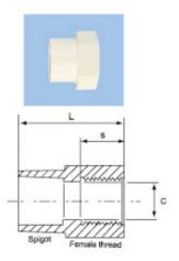
The spigot end of this fittings is solvent cement jointed to the socket of another fittings. The female threaded end provides a connection for male BSP threads such as spray nozzles.
