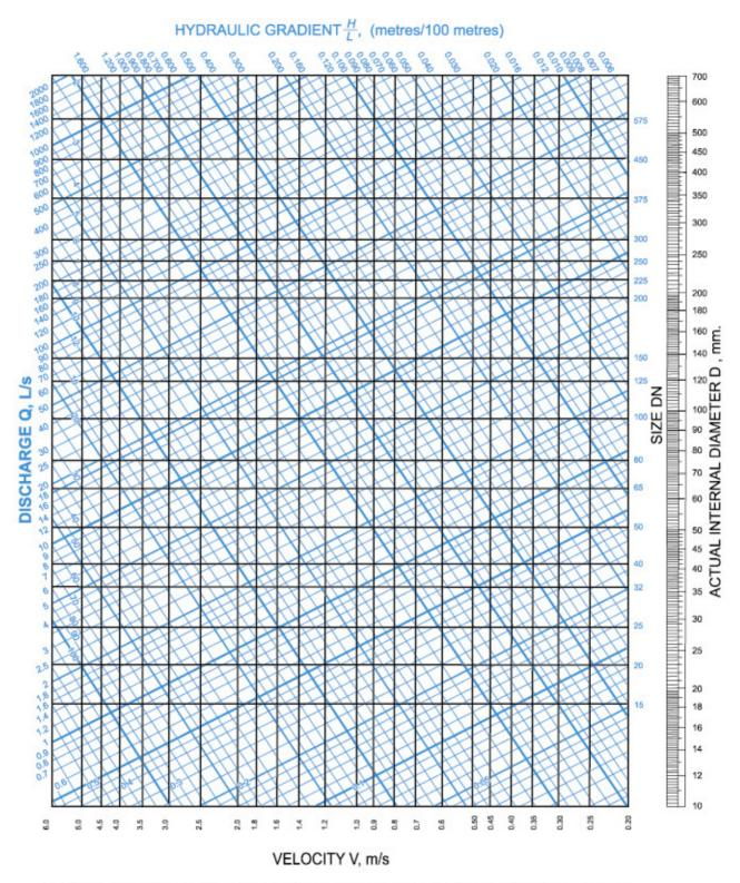
HYDRAULIC DESIGN OF PIPES k = 0.003mm BASED ON COLEBROOK-WHITE FORMULA FOP PIPES FLOWING FULL WITH WATER AT 20°C
