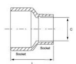
Reducing couplings are used for the solvent cement jointing of two different sizes of PVC pipe.
