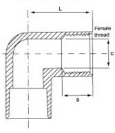
The faucet elbow is used to provide a female BSP connection. In irrigation it is used as a means of connecting a threaded riser pipe to an underground pipeline.
