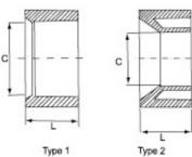
This fitting is used for solvent cement jointing into the socket of a fitting to give a reduction in bore.
