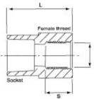
The faucet socket is solvent cement jointed to a pipe spigot. The femalethreaded end of the faucet socket provides a connection for a faucet tap fitting or a spray nozzle.
