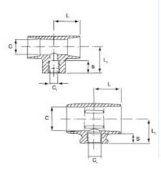
Faucet tees are used mainly in irrigation pipelines. The female thread in the tee branch provides a connection for a threaded riser pipe.
